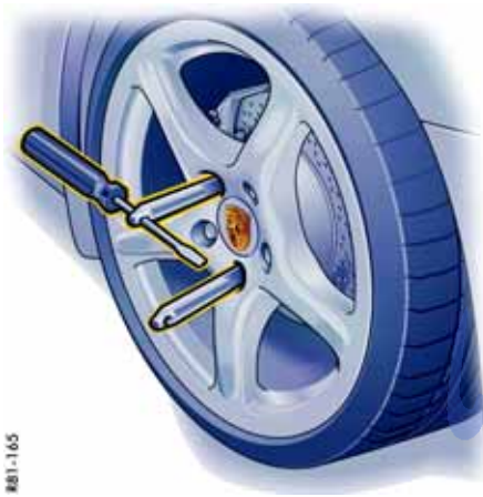
Screw in two assembly aids for vehicles with Porsche Ceramic Composite Brake
