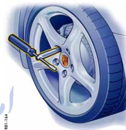
Screw in assembly aid for vehicles without Porsche Ceramic Composite Brake
