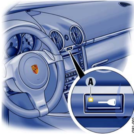
A - Light-emitting diode for alarm system
