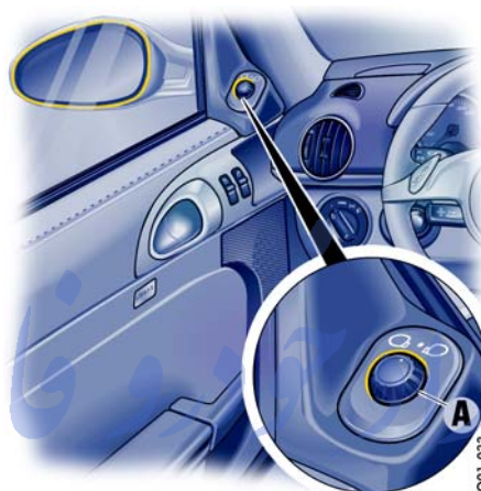
A - Control switch for door mirror adjustment
