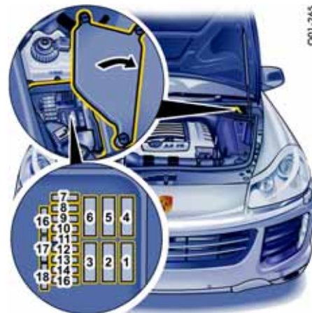
Fuse plan and fuse box in engine compartment
