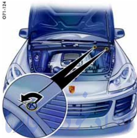
Cover of engine-compartment fuse box
