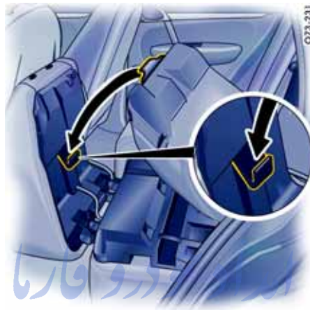
Rear seat assembly for comfort seats
