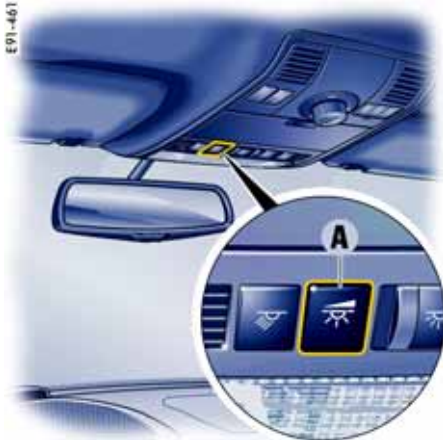
A - Button for dimming the comfort lighting
