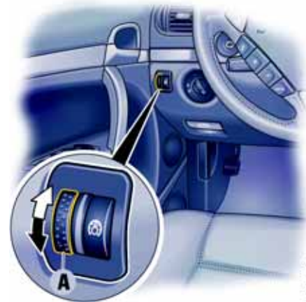
A - Instrument lighting knob
