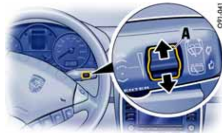
Rain sensor rotary switch
