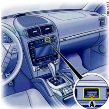
A - PASSENGER AIRBAG OFF indicator lamp
