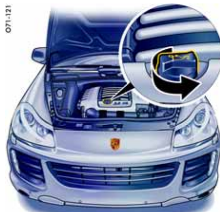
Engine oil filling point on Cayenne
