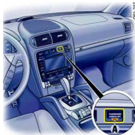
A - PASSENGER AIRBAG OFF indicator lamp
