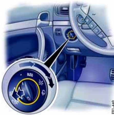
Light switch with driving light assistant
