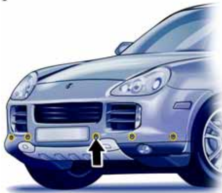
Front ultrasound sensors
