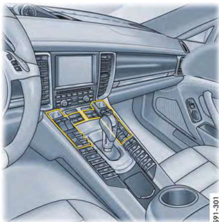
Front air-conditioning control panel
