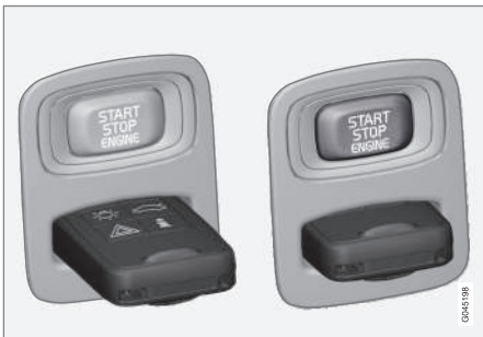
Ignition slot with remote key inserted (see Ignition modes (p. 79) for more information on ignition modes)
