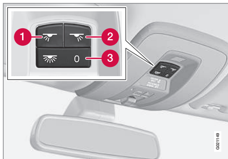
Light switches, front roof lighting
